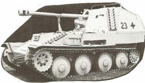
Marder III — AUSF M mounted on a Czech 38 (t) tank chassis.
